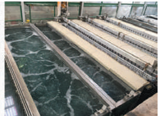
Profile anodising process
