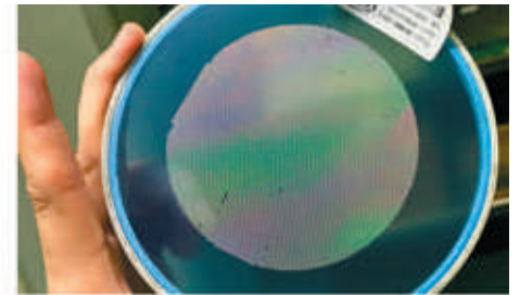
Base plate with more than 15.000 chips (diodes)
